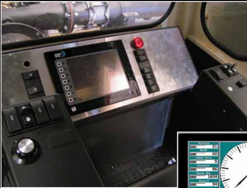
PLC based operating system with color touch screen interface
