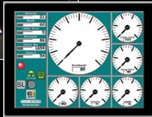
PLC based operating system with color touch screen interface
